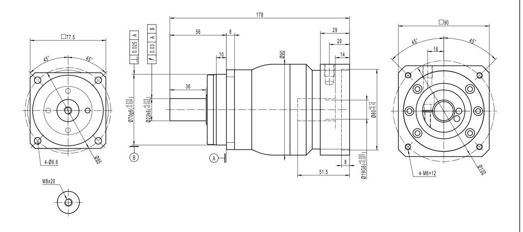
Note 1: This drawing shows the dimensions of X-Treme-SQ-ST-075 - 1 STAGE (this drawing is common to ratios 3 to 10)
