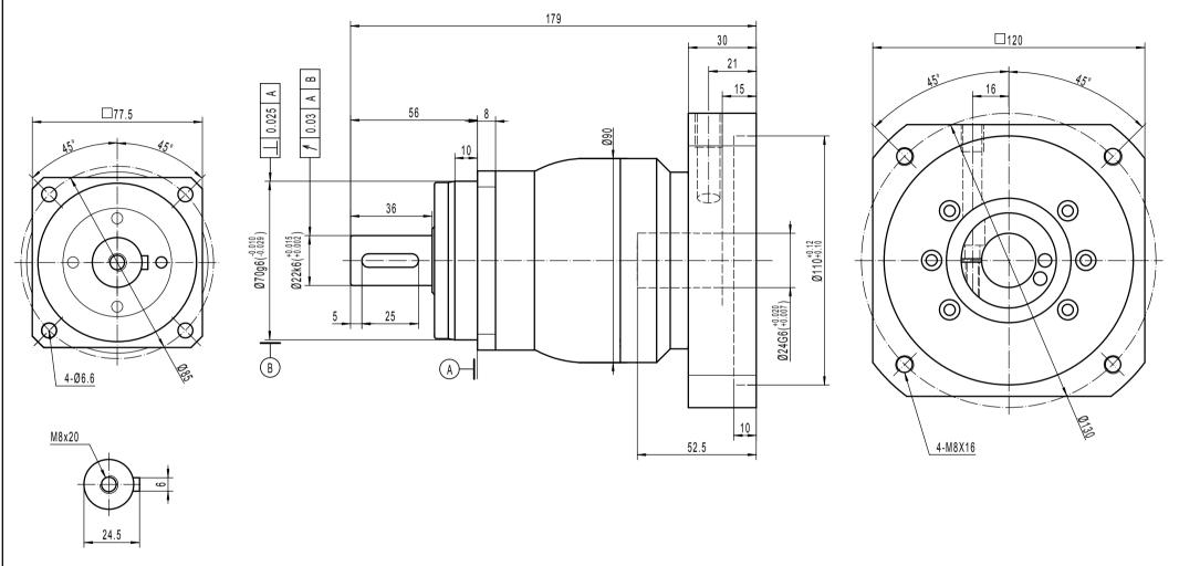
Note 1: This drawing shows the dimensions of X-Treme-SQ-ST-075 - 1 STAGE (this drawing is common to ratios 3 to 10)
