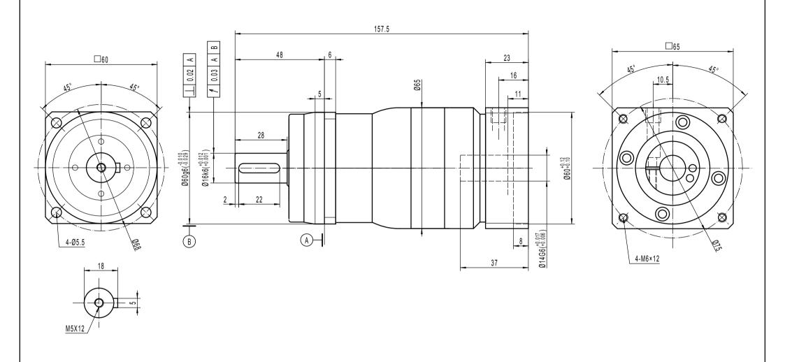
Note 1: This drawing shows the dimensions of X-Treme-SQ-ST-060 - 2 stages (It is common to all ratios from 12 to 100)
