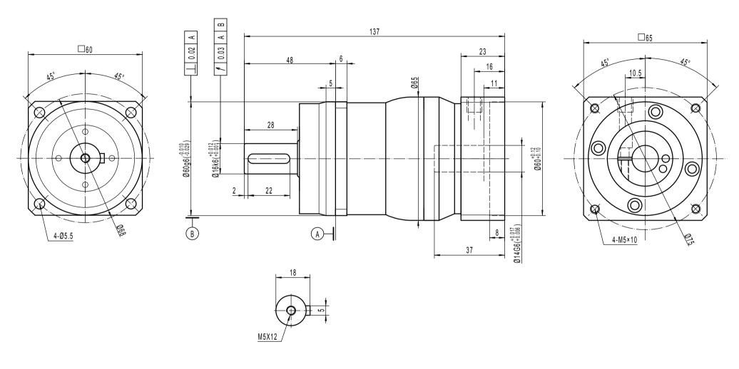
Note 1: This drawing shows the dimensions of X-Treme-SQ-ST-060 - 1 STAGE (this drawing is common to ratios 3 to 10)
