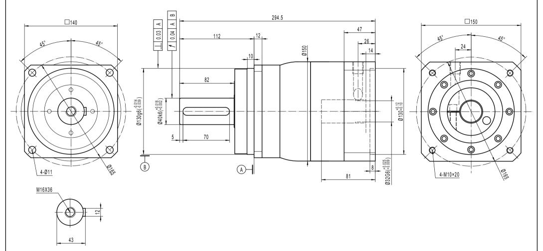
Note 1: This drawing shows the dimensions of X-Treme-SQ-ST-140 - 1 STAGE (this drawing is common to ratios 3 to 10)
