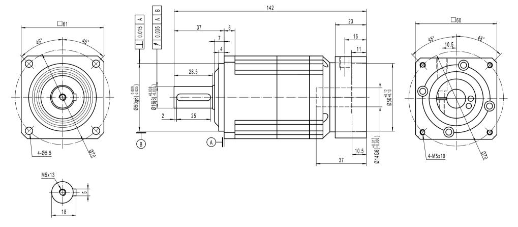
Note 1: This drawing shows the dimensions of WISER-SQ-ST-060 - 2 stages (It is common to all ratios from 12 to 100)
