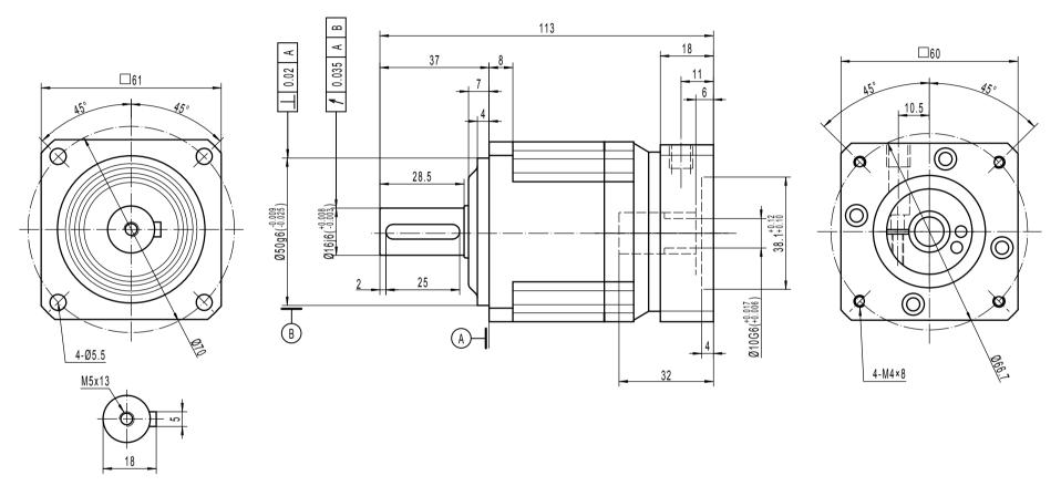
Note 1: This drawing shows the dimensions of Wiser-SQ-ST-060 - 1 STAGE (this drawing is common to ratios 3 to 10)
