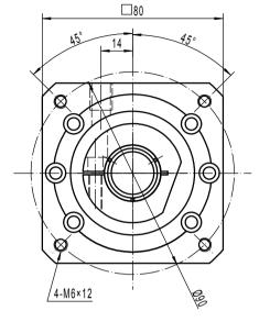
Note 1: This drawing shows the dimensions of Wiser-CI-ST-090 - 1 STAGE (this drawing is common to ratios 3 to 10)
