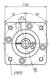
Note 1: This drawing shows the dimensions of Wiser-CI-ST-060 - 1 STAGE (this drawing is common to ratios 3 to 10)
