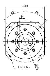
Note 1: This drawing shows the dimensions of ULTIMATE - CI - ST - 140 - 2 STAGES (this drawing is common to all ratios from 16 to 100)
