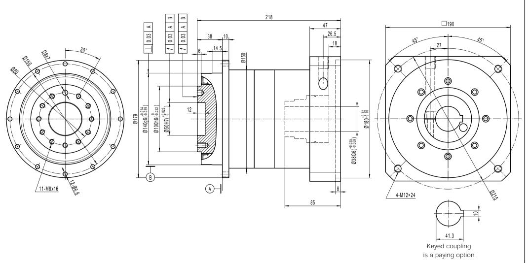
Note 1: This drawing shows the dimensions of ULTIMATE-CI-ST-140 - 2 STAGES (this drawing is common to all ratios from 16 to 100)
