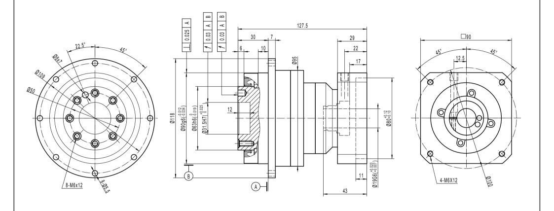
Note 1: This drawing shows the dimensions of ULTIMATE - CI - ST - 090 - 2 STAGES (this drawing is common to all ratios from 16 to 100)
