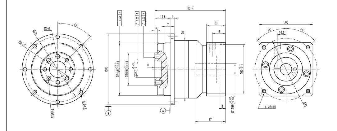
Note 1: This drawing shows the dimensions of ULTIMATE-CI-ST-064 - 1 STAGE (this drawing is common to all ratios from 4 to 10)
