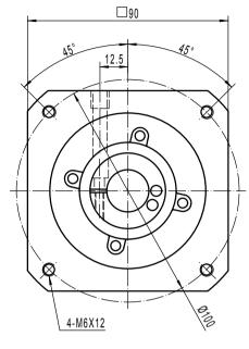
Note 1: This drawing shows the dimensions of LIVELY-SQ-ST-090 - 2 stages (It is common to all ratios from 12 to 100)
