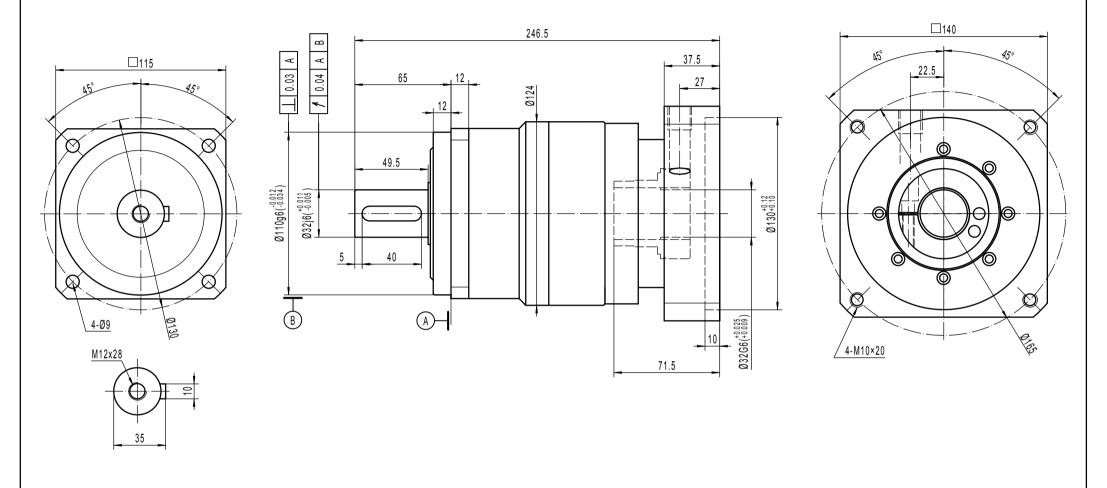
Note 1: This drawing shows the dimensions of BOOSTER-SQ-ST-120 - 2 stages which are common to all ratios from 12 to 100)
