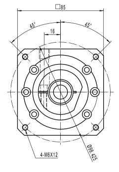
Note 1: This drawing shows the dimensions of BOOSTER-SQ-ST-090 - 1 STAGE (this drawing is common to ratios 3 to 10)
