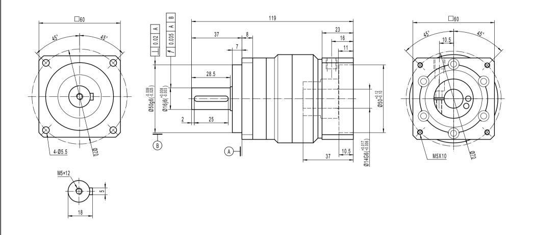
Note 1: This drawing shows the dimensions of BOOSTER-SQ-ST-060 - 1 STAGE (this drawing is common to ratios 3 to 10)
