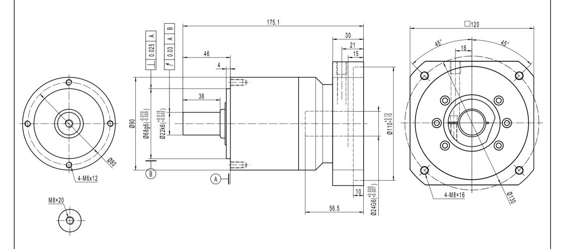
Note 1: This drawing shows the dimensions of ACCESS-CI-ST-090 - 1 STAGE (this drawing is common to ratios 3 to 10)
