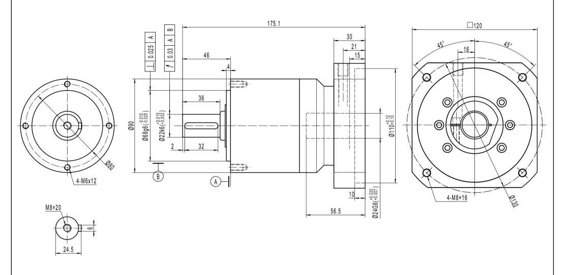
Note 1: This drawing shows the dimensions of ACCESS-CI-ST-090 - 1 STAGE (this drawing is common to ratios 3 to 10)
