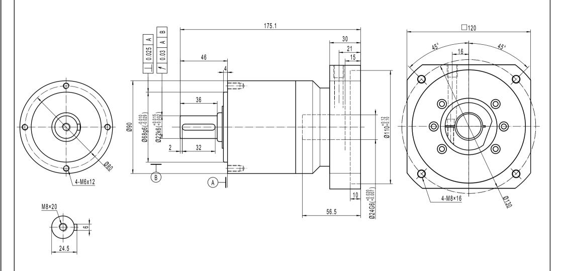
Note 1: This drawing shows the dimensions of ACCESS-CI-ST-090 - 1 STAGE (drawing common to ratios 3 to 10)
