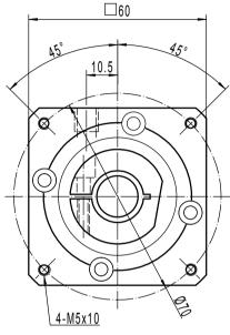
Note 1: This drawing shows the dimensions of ACCESS-CI-ST-070 - 1 STAGE (this drawing is common to ratios 3 to 10)
